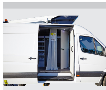
Walk-Through-System: Direct access from the cabin to the bucket through the vehicle (optional)
